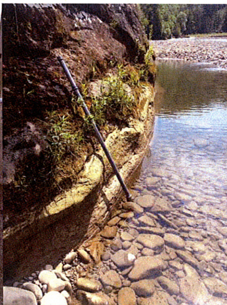
Montage Temperatur- logger
